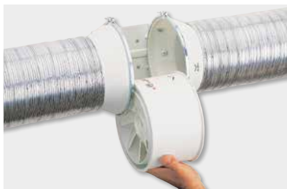
The unique design of the support bracket allows the motor and impeller assembly to be fitted or removed without dismantling the adjacent ducting.
