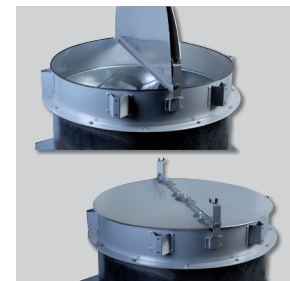
Back draft shutter Prevent back draft of air and entrance of rain water when the fan is switched off.
